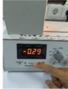
Figure 4. Changing the Display Mode to Voltage Mode.
