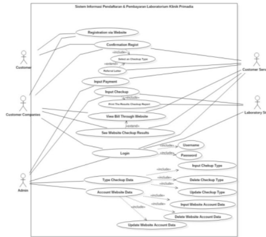
Fig. 4. Use Case Diagram of Proposed System
